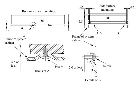
Figure 3.5 Mounting frame structure
